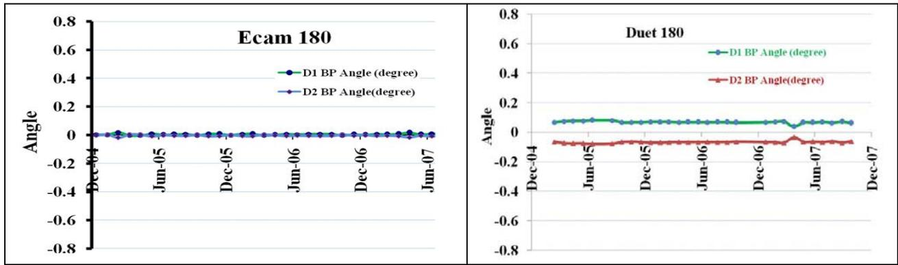
**Fig. 11.** The Back projection angle result for detector 1 (D1) and detector 2 (D2) in Ecam camera with 180 configuration degrees through 30 months.
