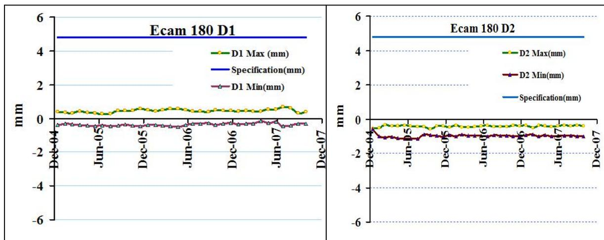
**Fig 3:** MHR/ COR calibration result of X- Maximum, X- minimum and specification for detector 1(D1) and detector 2 (D2) in Ecam camera with 180 configuration degree through 30 months.
