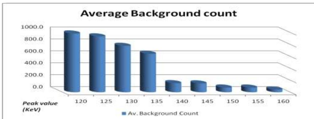
**Figure (2):** Relationship between the changes in the peak energy with the average background counts for the measured sphere with the same size.
