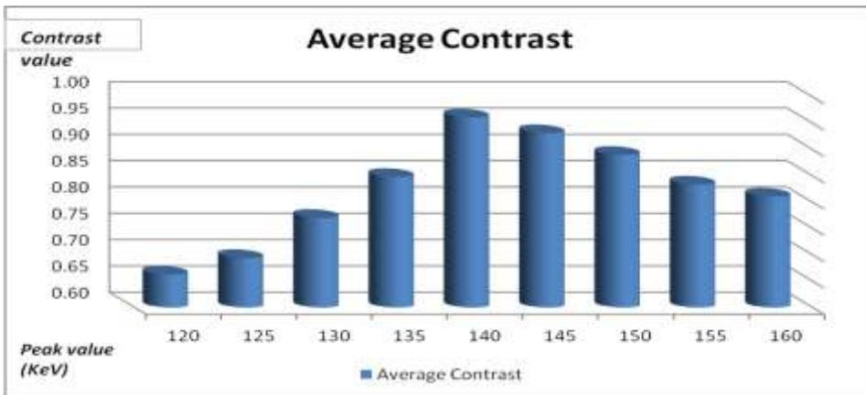
**Figure (3):** Relationship between the changes in the peak energy with the average contrast value for the measured sphere.
