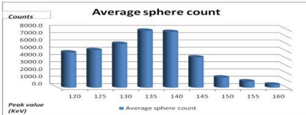
**Figure (1):** Relationship between the changes in the peak energy with the average counts in the measured sphere.
